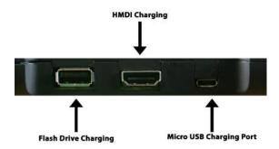
USB Port – Used to attach a flash drive to the UbiDuo 2. This provides a way to copy saved conversations or to install firmware upgrades.
