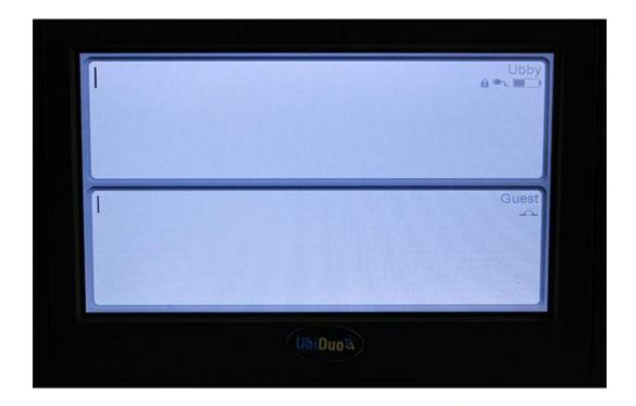
Both halves of the UbiDuo 2 must be turned on for a split screen chat to be initiated. The two halves will automatically connect with each other when the split screen chat is selected on one of the halves.
