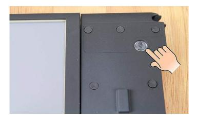
To turn off the UbiDuo 2, press and release the power button. If any existing conversations have not been explicitly saved, turning the UbiDuo 2 off wipes them from the device's memory.
