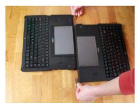
To separate the two halves of the UbiDuo without damaging the internal parts, always lay the UbiDuo flat preferably on a hard surface such as a desk or table. Then grasp the J-hook technology and pull them away from each other.
