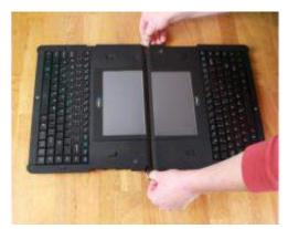
To connect the two halves, lay the UbiDuo flat on a desk then connect them by using the J-hook technology to pull them back together using the plastic cases. The joint cover has to line up straight.
